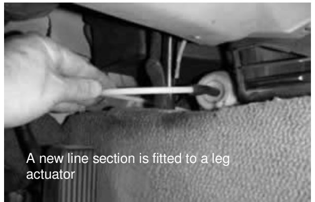
A section of leaking line can be cut and replaced
