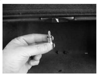
The glove box light can be removed by inserting a thin screwdriver edge at the front then gently prying down and toward the rear. When the light is removed from its hole the glove-box liner may be removed.
