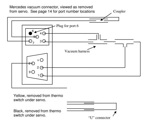
This configuration connects port 7 with port 5 to open the Center Vent. Leave port 8 open to close the leg vent.
