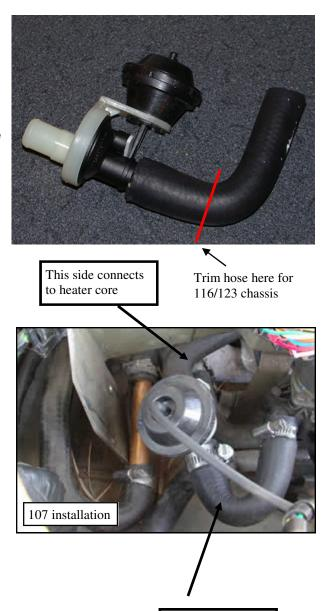
Water Valve This side connects to aux water pump
