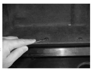
Next remove the 2 screws which hold the glove box latch in place. These screws are oriented vertically and there is little clearance. A very short screwdriver or a 1/4" ratchet drive screwdriver will be needed.
