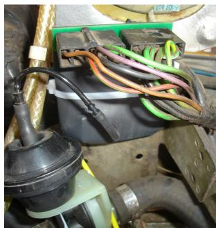
Mercedes Servo Connector 10 pins, 1/4" female fast-ons Embedded in 2 plastic housings
