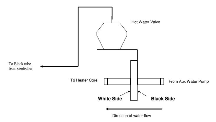
Note: The Black side MUST face toward the auxiliary water pump. If this valve is installed backward it will not turn completely off!
