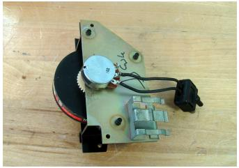
Set the thumbwheel for 75 degrees and rotate the body of the potentiometer so that that the resistance of the thumbwheel is 900 ohms, +/-50 Ohms at a dial setting of 75 degrees. Now tighten the nut on the potentiometer.
