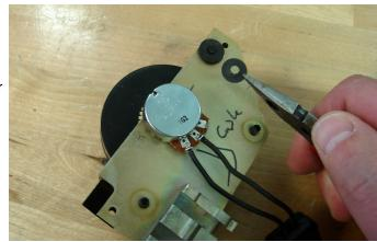
Note: this version of the kit uses a slightly higher value of potentiometer than the stock part. The value is now 2500 ohms instead of 2000 ohms. This gives you a slightly cooler setting in summer, with longer max cool, and slightly warmer in winter. The value at 75 degrees is calibrated.
