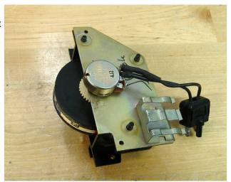
Now remove the metal side-plate with the attached potentiometer. Remove the potentiometer.
