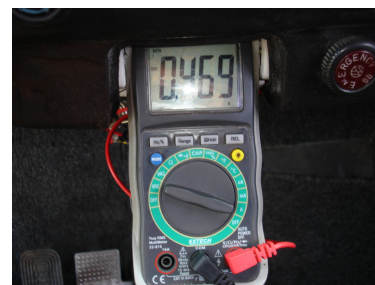
Volt meter reading oxygen sensor in volts
