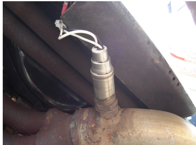
Bosch 13913 sensor installed in bung welded to header
