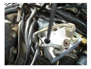
Now tighten the fuel fittings on the top of the valve assembly then tighten the fuel lines. Note: The fuel lines must be properly torqued, not over-torqued, to prevent leaks. Use a backing wrench as shown to properly tighten the fuel line nut onto the fitting. The body of the UTCIS<sup>™</sup> is aluminum, DON'T STRIP THE THREADS!!
