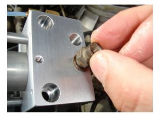
The body of the UTCIS<sup>™</sup> regulator can now be mounted in the same location as the OEM part. The aluminum spacers in the hardware kit are used to position the UTCIS<sup>™</sup> at the same height as the OEM regulator. Tighten the M6 x 65 mm screws as shown. These screws thread into the same mounting points as the OEM Warmup Regulator.
